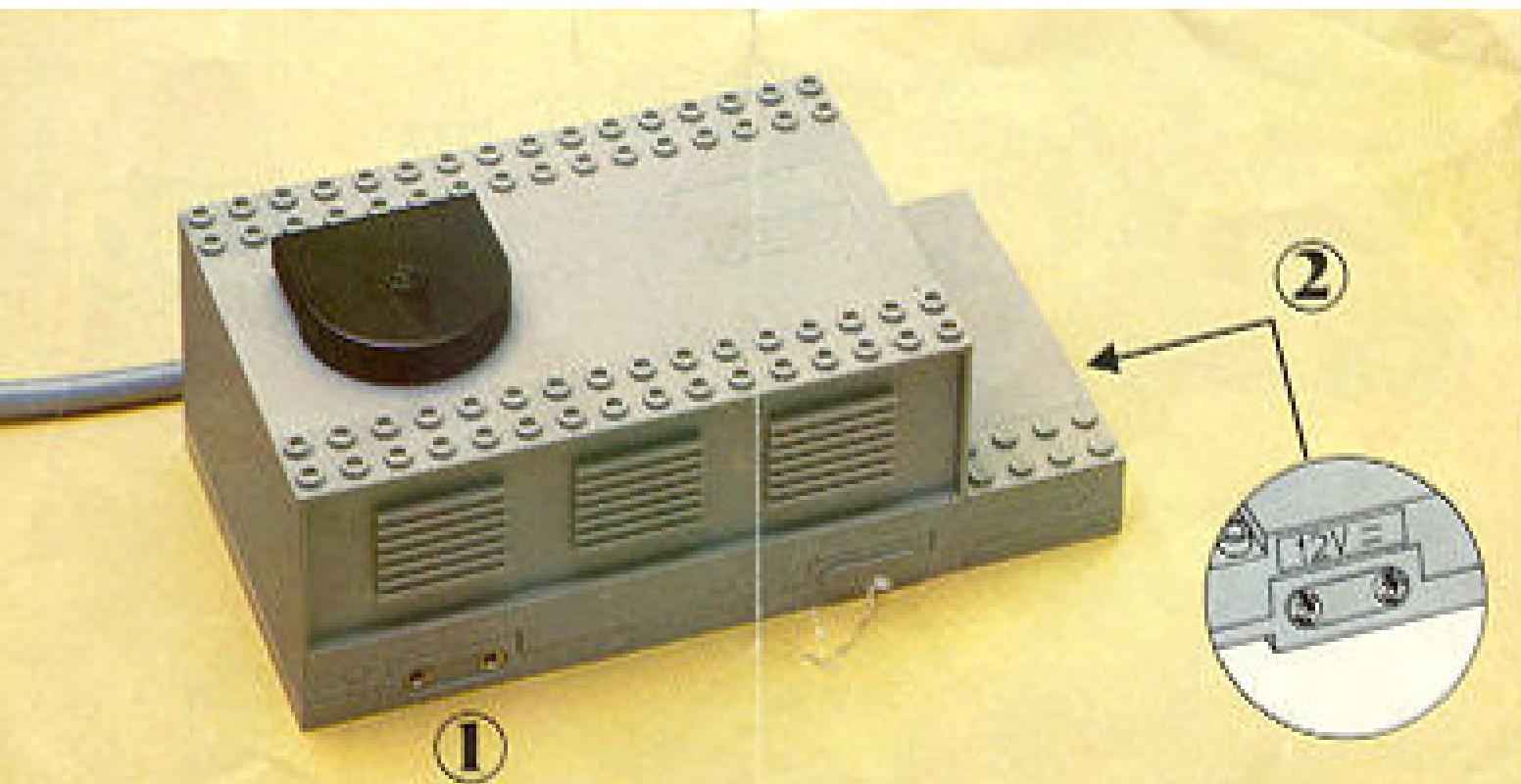
**1.** 0 - 12 volt DC variable outlet. Supplies current to the rails of the Electric Railway or Technical motor 880.
